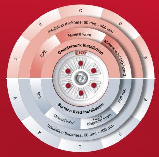
We invented the EJOT STR principle to create the perfect, homogeneous insulating surface. The safe fastening of the insulation is achieved in four quick and simple steps, resulting in a barely visible fixing:
